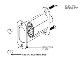
Note: Through Bolt Mount Kit is for 3/4" maximum material thickness.
