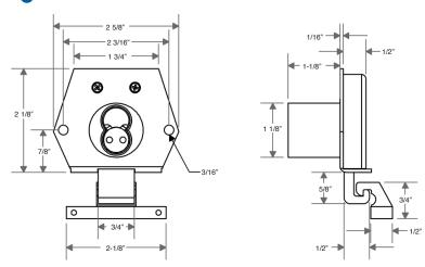
MORTISE MOUNT INVERTED INTERLOCKING SPRING BOLT
