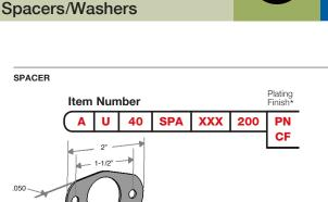
Made in the U.S.A For use with D, K, K2, M, S, V and E40 Plunger Locks.
